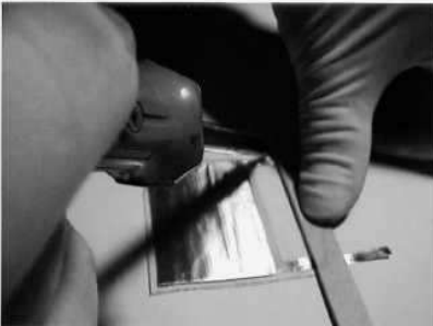
Sealing plastic with solder-iron
