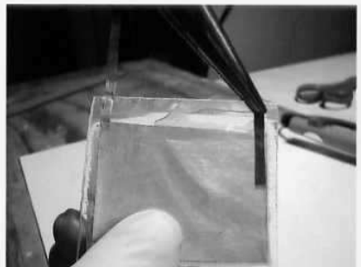
Bending back metal contacts
